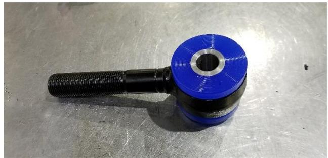
4. Measure the length of the factory toe arm and make the RalliTEK toe arm the same length.
