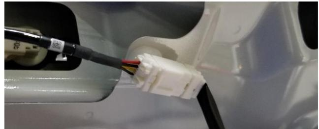
5. Route the light wire harness through the hatch, I used the same grommet that the reverse camera wires go through
