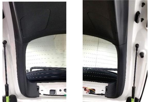
3. Some models may have a clip that holds the rear panel on, remove that at this time and gently pull straight off the hatch, it helps to start at one corner and work your way over to the other side
