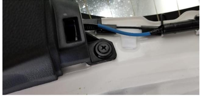
4. Remove the 4 nuts that hold the rear exterior trim piece to the hatch (2 are easy to see and the other 2 can be accessed through holes in the inner structure), unplug the wire harness and pull straight out on the trim piece to remove
